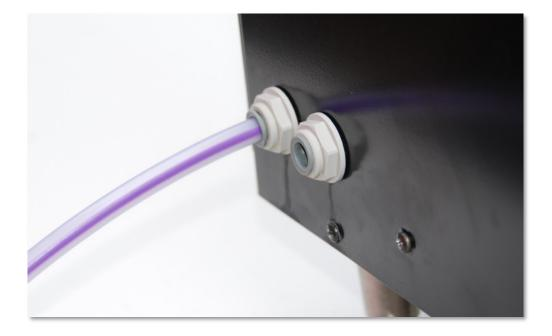
Locate the John Guest fitting located on the lower right corner of the back of the dispenser.
