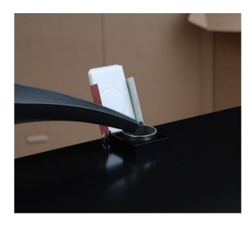
Open tank door on the top of the machine and add approximately 1 and ½ gallons of water until water level is just below the bottom of the filling cylinder. DO NOT OVER FILL!!!
